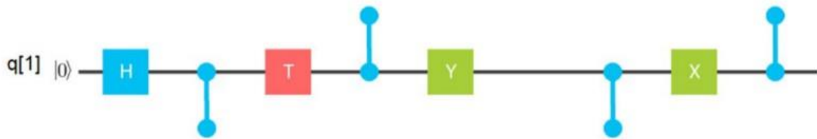
(b) The "bristle-brush" pattern formed by the gates applied to qubit q[1]
